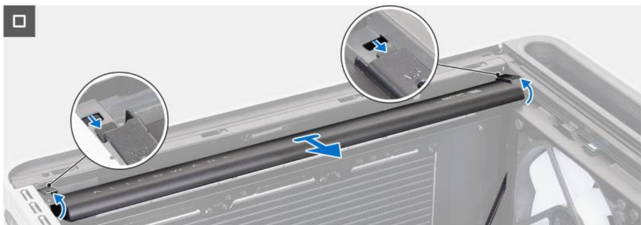
Figure 71. Removing the side light
