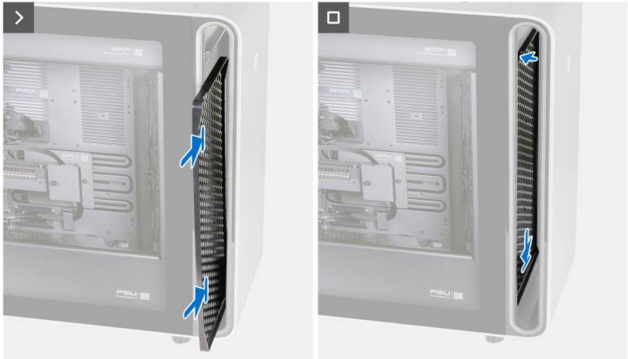
Figure 31. Installing the front fan filter
