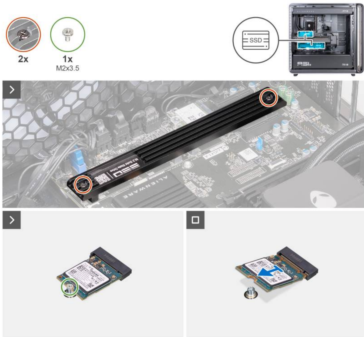
Figure 40. Removing the M.2 2230 SSD
