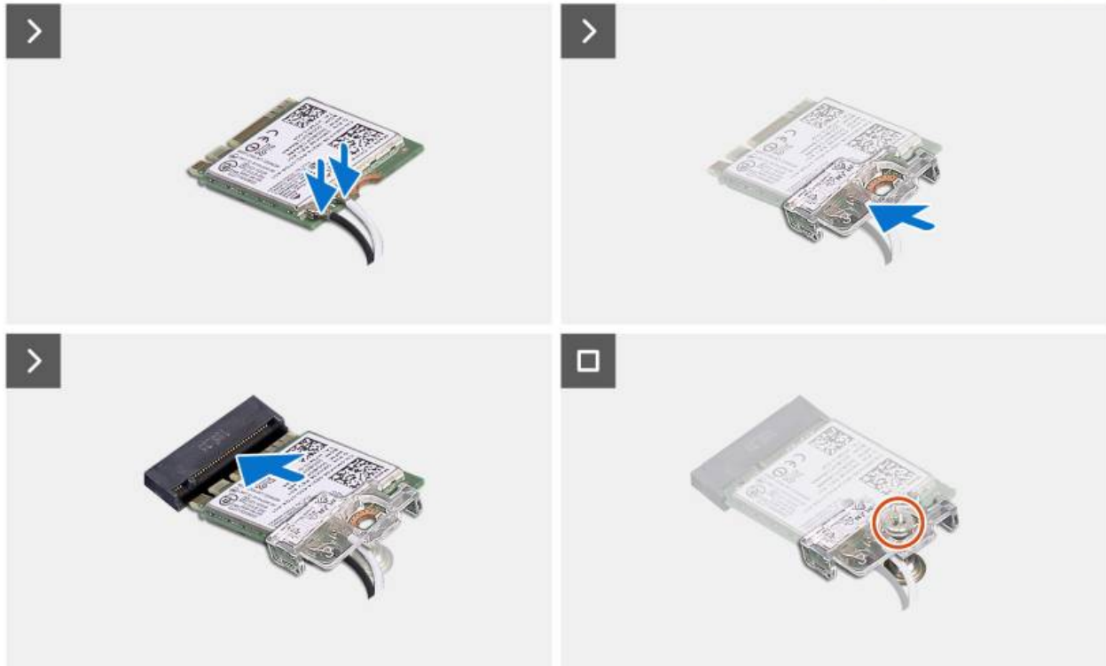
Figure 47. Installing the wireless card
