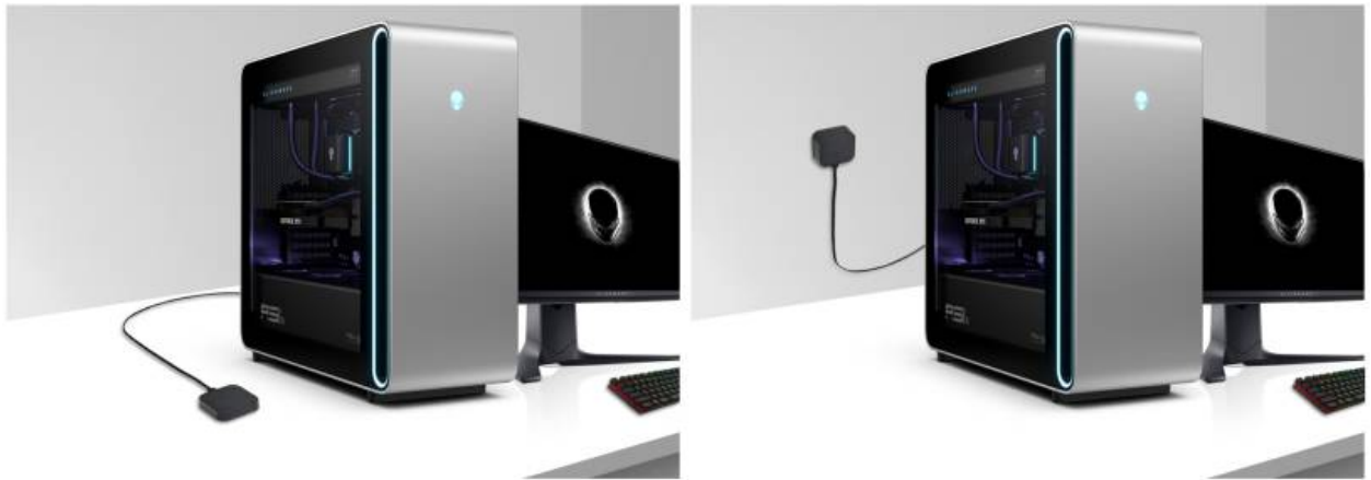
Figure 13. Placing the antenna in a suitable location
