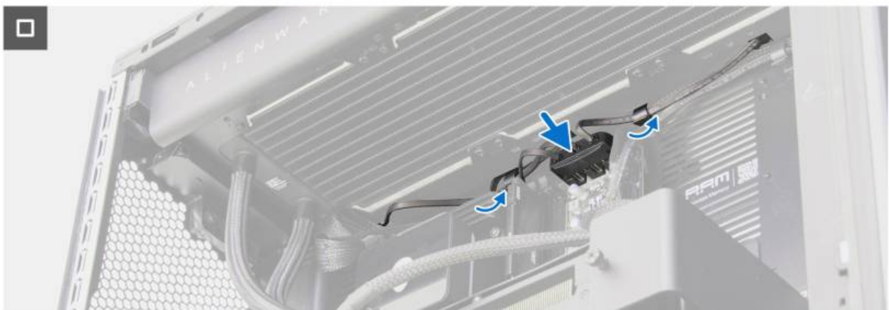
Figure 81. Installing the top fan
