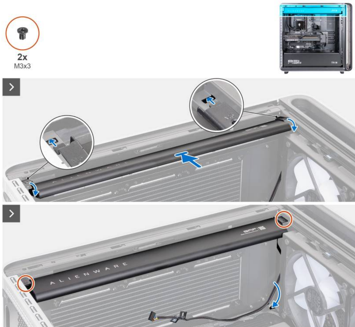
Figure 72. Installing the side light
