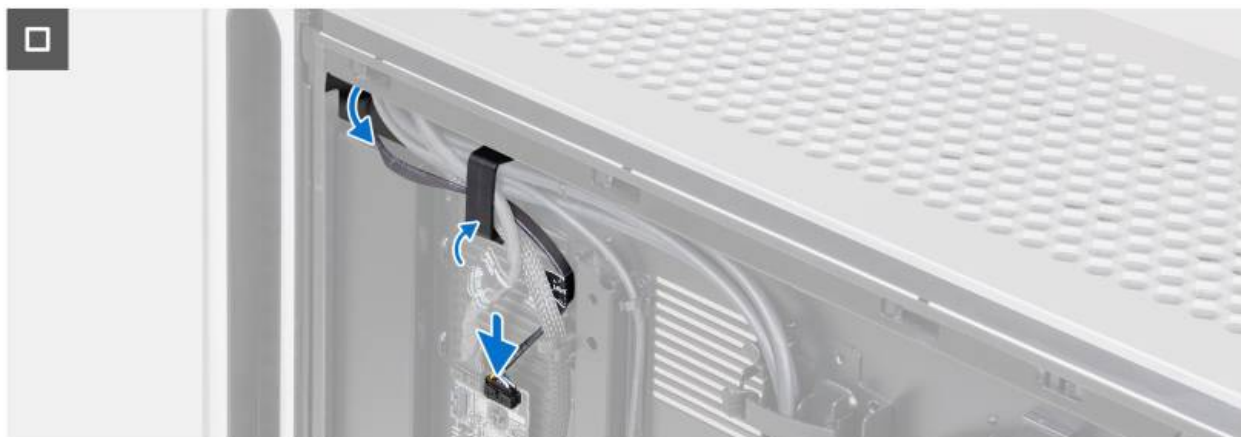
Figure 73. Installing the side light
