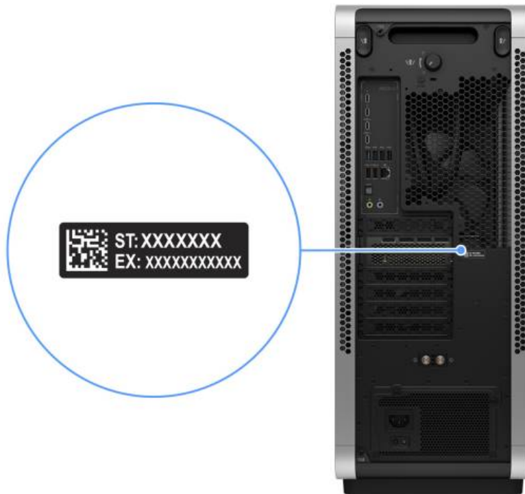
Figure 5. Service Tag/Express Service Code location
