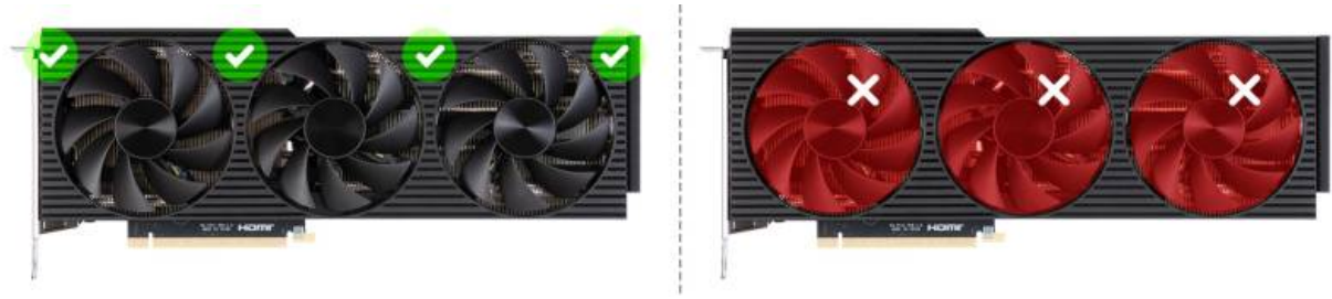
Figure 37. Right location to hold the graphics card
