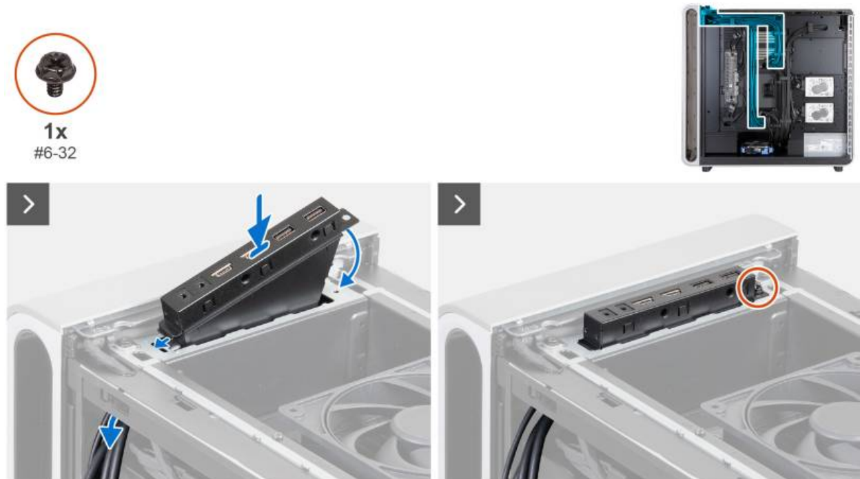
Figure 66. Installing the top I/O-panel
