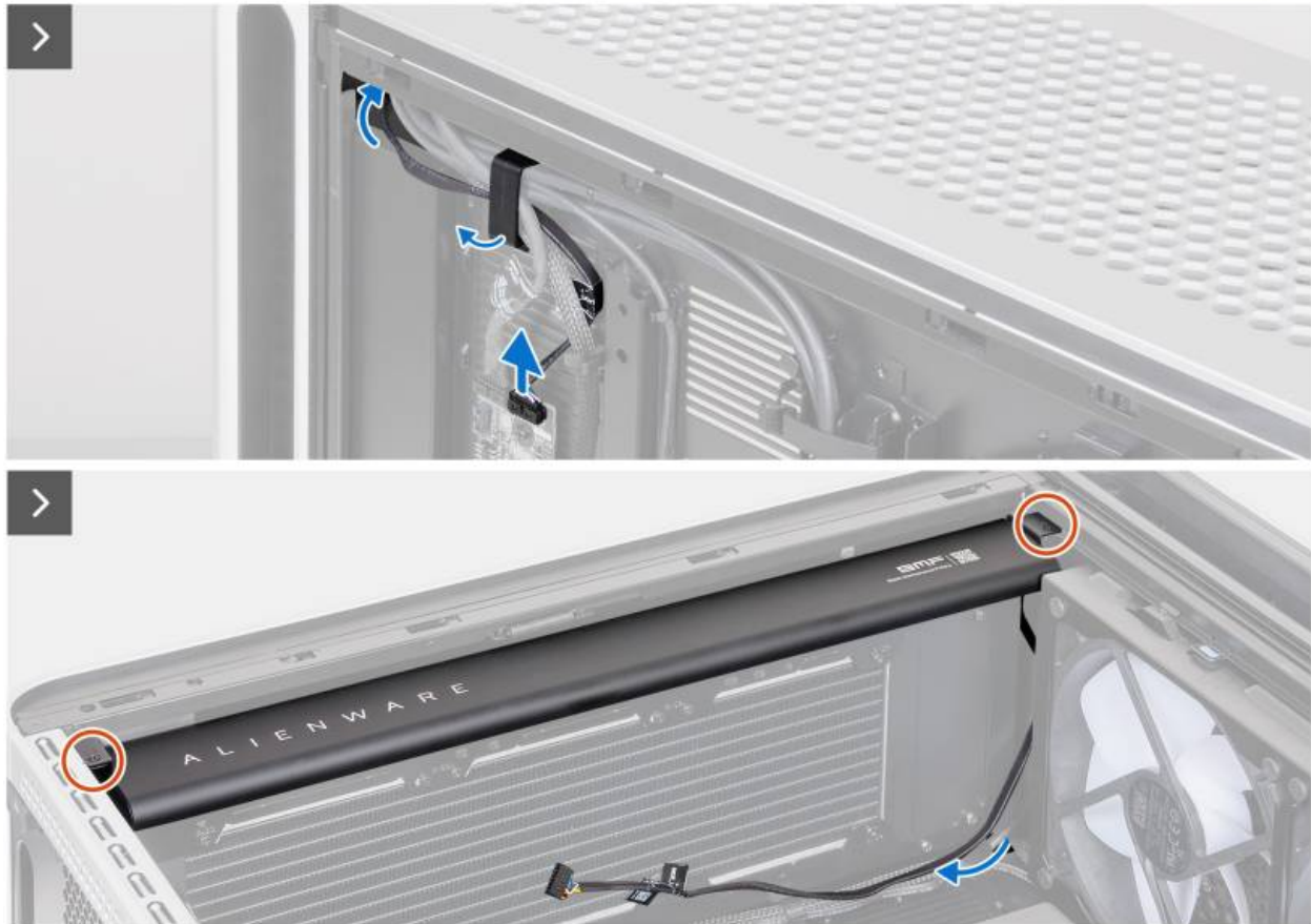
Figure 70. Removing the side light
