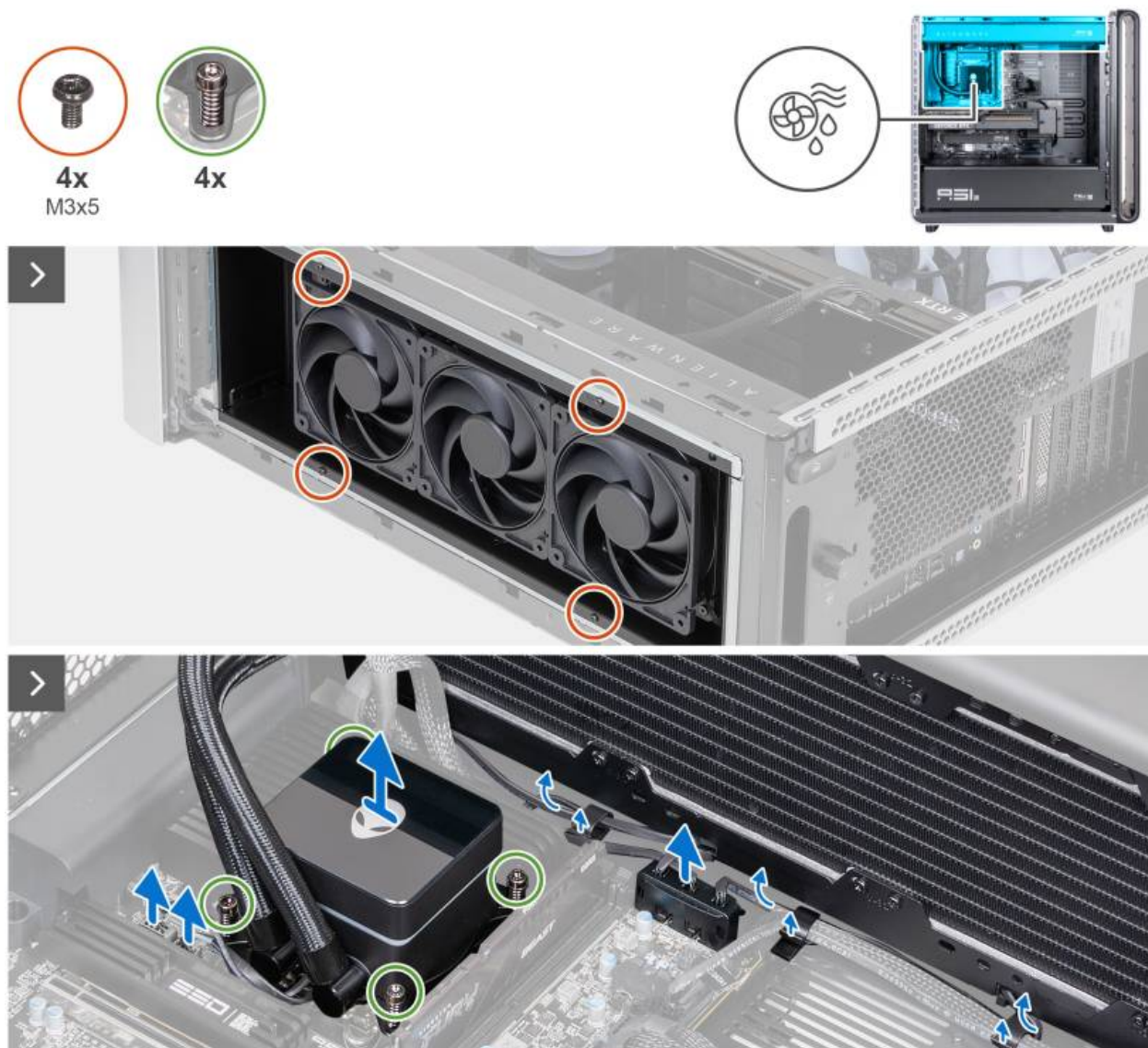
Figure 74. Removing the processor liquid-cooling assembly
