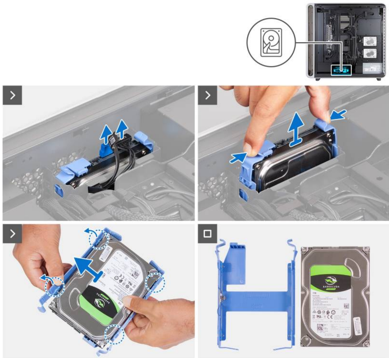
Figure 62. Removing the 3.5-inch hard drive
