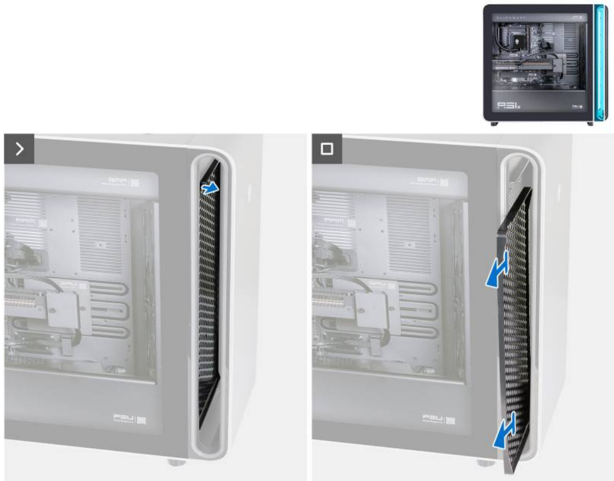
Figure 30. Removing the front fan filter
