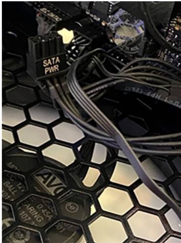
Figure 23. Do not connect the SATA PWR and the ELC DATA1 cables that were shipped along with your computer to the motherboard.
