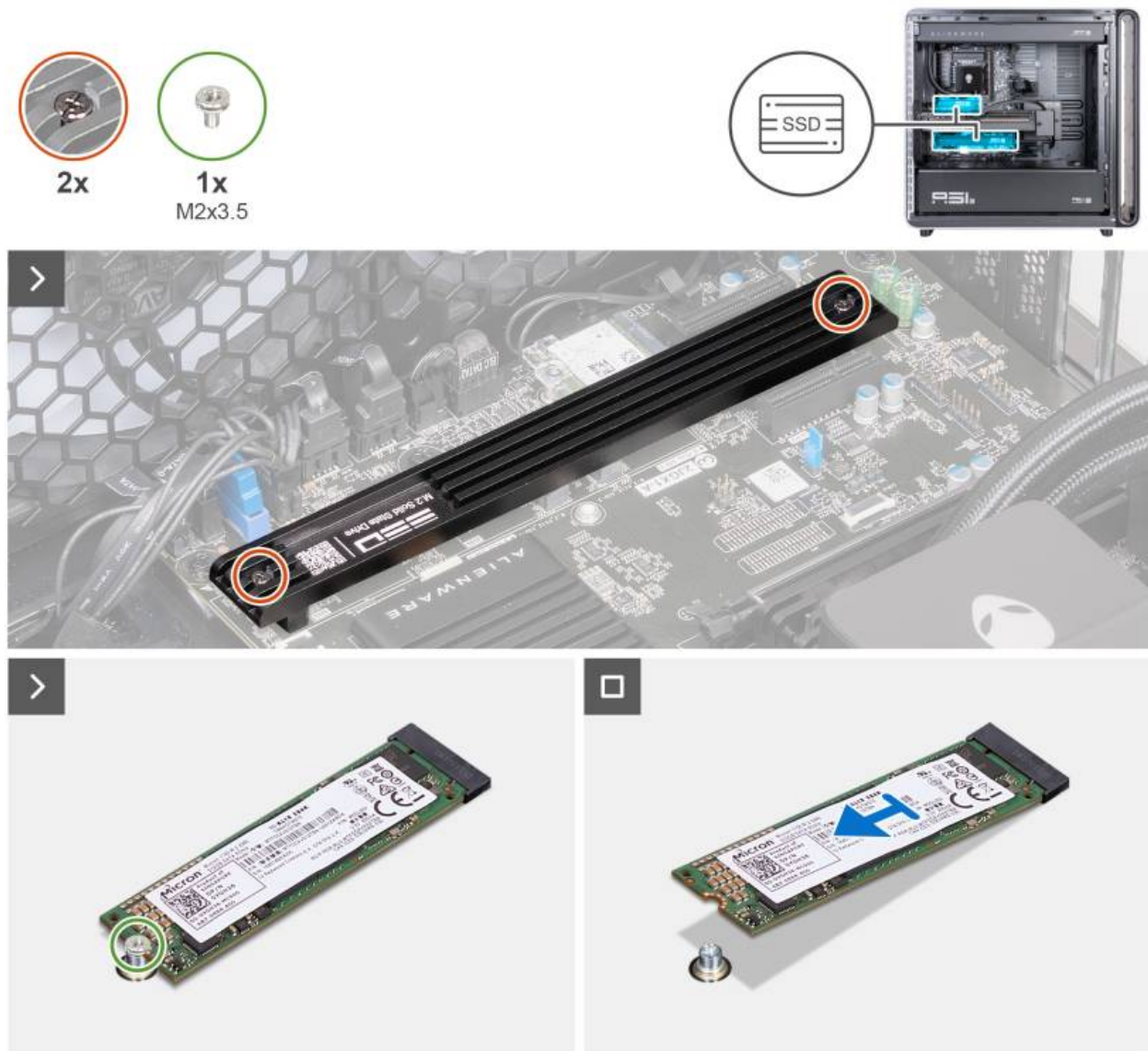
Figure 43. Removing the M.2 2280 SSD
